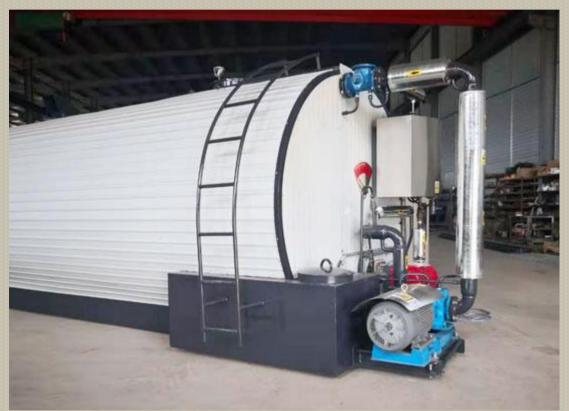
The oil heating bitumen tank adopts world famous brand oil burner, which is high efficient and environmental friendly. The combustion is sufficient and steady. Target temperature can be pre-set and the machine will perform the rest work (machine will auto shut down once reaching the upper limit, and will auto start when reaching bottom limit).
