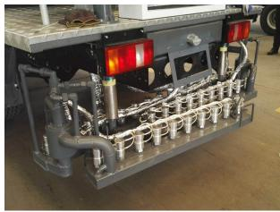
.Asphalt pump: which has good pumping capacity, large discharge capacity, can do a better performance of asphalt circulation and spraying.
