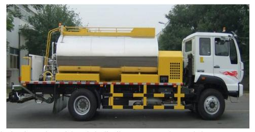
Asphalt distributing is used special asphalt distributor to spray hot asphalt on pavement on the basis of measured distributing amount and pressure. It is mainly used deal with the construction of upper and lower seal coat, prime layer, asphalt surfacing, asphalt penetration surface, fog seal layer and so on.
